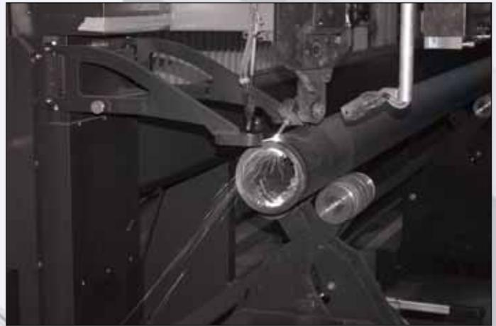
Our 2 Wernet Behringer band saws and MAP punching and shearing machine make it possible to cut all standard EURO profiles. Drill holes are prepared by a 3-spindle FP1215 drill that allows us to drill each side of the EURO profiles without re-clamping.
