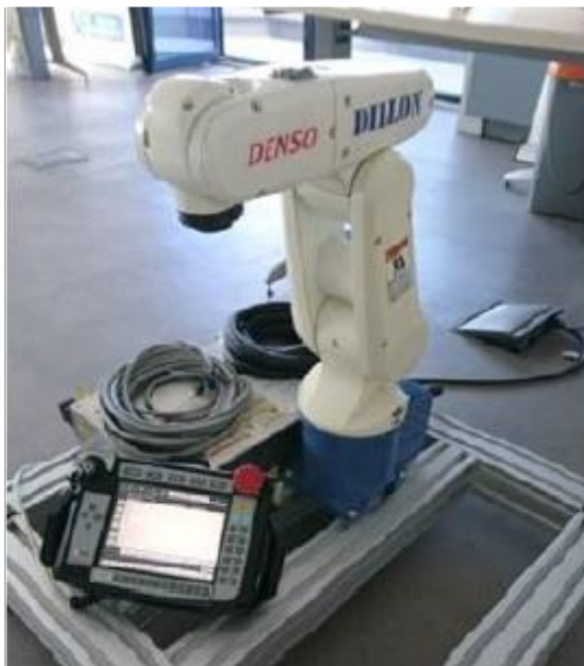
Figure 22 Robots used in experimental validation[12]. (left) Denso VP-6242 robot used of offline and online testing. (right) ABB IRB120 robot which was used in online testing.
