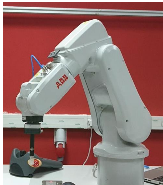
Figure 22 Robots used in experimental validation[12]. (left) Denso VP-6242 robot used of offline and online testing. (right) ABB IRB120 robot which was used in online testing.
