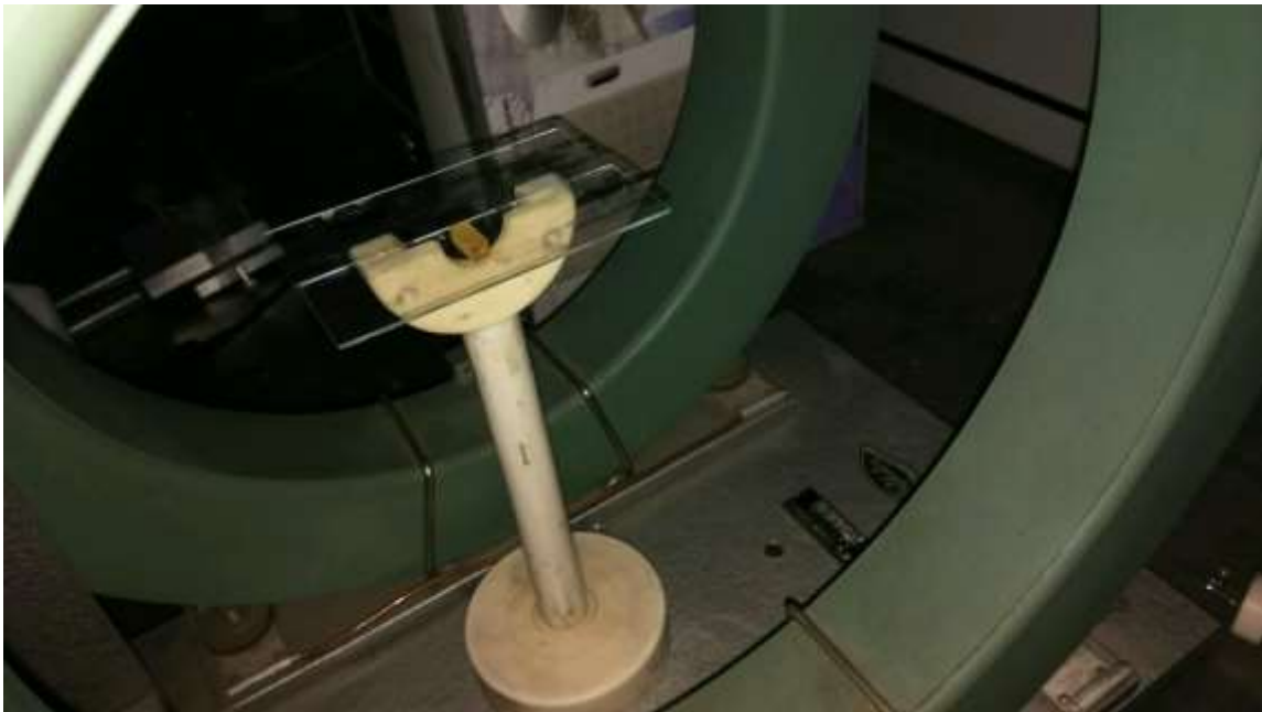
Figure 36 The mounting setup used to suspend the crystal in the Helmholtz coils magnetic field.
