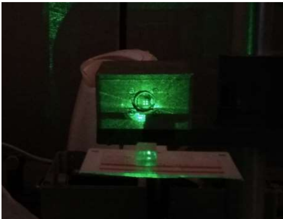
Figure 42 Laser beam spots on the photodiode detector following the beam splitting process.
