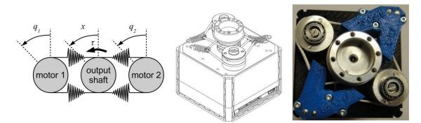
Figure 1.17. Functional scheme of bidirectional antagonistic drive employed in qbmove maker pro actuator designed by QB Robotics; (middle) Schematic of qbmove maker pro actuator (left); Prototype of low-cost qb move maker pro actuator, most of whose parts could be built using a 3D printer (right).
