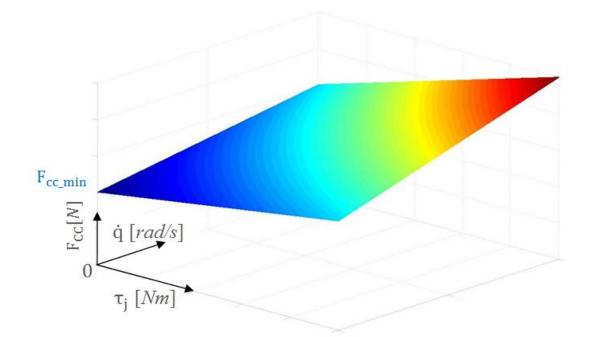
Figure 5.3. Desired force in the antagonist tendon of the i-th joint, estimated using a bio-inspired torque share algorithm. Reference tension force rises with increase in desired net joint torque (corresponding to biological reciprocal activation) and increase in joint velocity.
