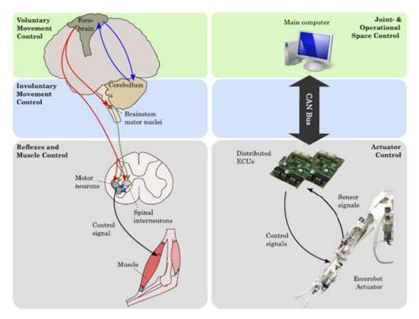
Figure 1.6. Example of distributed control architecture that seeks to resemble its biological paragon in humans. Electrical control units (ECUs) are used for low-level actuator feedback loops, mimicking reflex arcs that are closed through the spinal cord, while a high-level central processor unit acquires all sensory data and commands motion planning via a controller area network that emulates the central nervous system.
