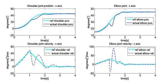
Figure 3.24. Puller-follower control applied to a 2-DoF robot arm actuated by antagonistic compliant drives. The top two windows depict shoulder and elbow positions, and the bottom windows show velocities during movement in the vertical plane. Trajectory tracking demonstrates how puller-follower control deals with a multi-joint system, nonlinearities caused by gravity, changeable effective joint inertia, and external disturbances (impact with an external object at t = 1s).
