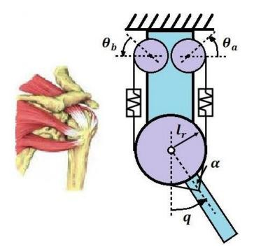
Figure 2.4. Demonstration of a human joint with constant moment arms (shoulder joint) - (left); Circular joint structure as a classical scheme of antagonistic joints with constant moment arms (right). This model is suggested as an approximation for shoulder or knee joint modeling.
