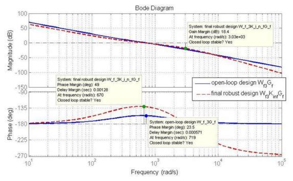
Figure 3.22. Contributions of  $H_{\infty}$  optimization to robust stability enhancements of the target system: lowered open-loop gain at high frequencies and improved stability margins. The frequency characteristics of the antagonistic force subsystem already shaped by the pre-compensator  $W_{f3} - W_{f3}G_f$  (solid blue line), is improved using the  $K_{\infty}_{F3}$  robust stability compensator  $-W_{f3}K_{\infty}_{F3}G_f$  (dashed red line).
