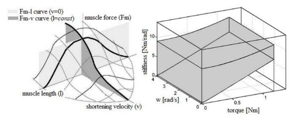
Figure 1.4. Force-length-velocity 3D plot of a human muscle as a biological paragon of variable stiffness actuators – VSAs (left); Torque-stiffness-velocity 3D plot of achievable characteristics of a qbmove actuator as a VSA representative (right).
