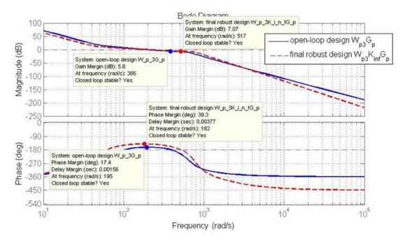
Figure 3.23. Contributions of  $H_{\infty}$  optimization to robust stability enhancements of the target system: lowered open-loop gain at high frequencies and improved stability margins. The frequency characteristics of the joint position subsystem already shaped by the pre-compensator  $W_{p3} - W_{p3}G_p$  (solid blue line) is improved using the  $K_{\infty}_{P3}$  robust stability compensator  $-W_{p3}K_{\infty}_{P3}G_p$  (dashed red line).
