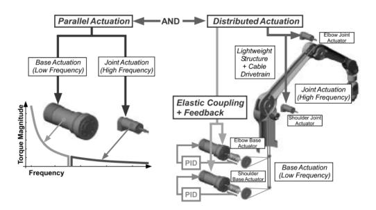
Figure 1.9. DM<sup>2</sup> approach: torque partition among low-frequency high-torque and highfrequency low-torque actuators, contributing in parallel to overall joint torque (left); Actuator distribution: large, low-frequency actuators are tendon driven SEA located at the base to reduce effective inertia, whereas small, high-frequency actuators are located at the joints to enable high bandwidth control (right).
