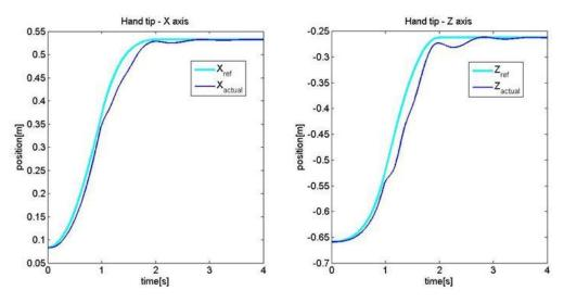
Figure 3.25. Puller-follower control applied to a 2-DoF robot arm actuated by antagonistic compliant drives. Horizontal (left window) and vertical (right window) Cartesian coordinates demonstrate the effects of gravity compensation, effective joint inertia and impact in the vertical plane.
