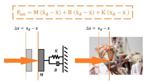
Figure 5.1. Impedance control principle. A robot controlled by an impedance controller behaves as a second order mass-spring-damper system in Cartesian space.
