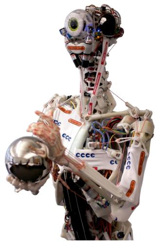
*Figure 2.2. Eccerobot – an upper-body anthropomimetic robot. This prototype served as the target system for modeling of a typical anthropomimetic robot.*
