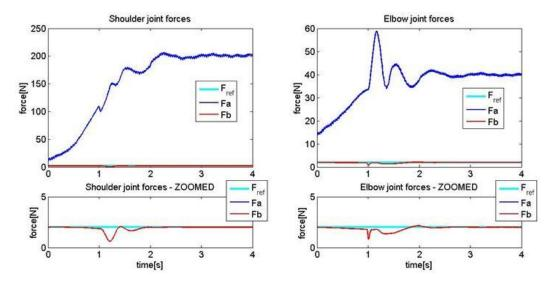
Figure 3.26. Puller-follower control applied to a 2-DoF robot arm actuated by antagonistic compliant drives. Agonist and antagonist tendon forces in shoulder and elbow joints during movement in the vertical plane (top windows); Zoomed in detail from the top – force tracking in antagonist tendons. Both antagonistic tendons remain tight even though impact occurs (bottom windows).
