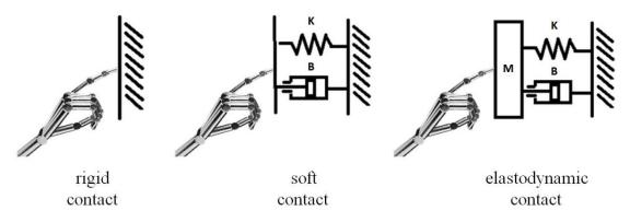
Figure 2.9. Division of contacts according to the type of elastic deformations in the contact zone.
