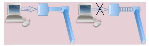
Figure 1.3. Basic principle of active compliance – compliant joint behavior is purely a result of software action (left) and passive compliance – compliant joint behavior is a result of mechanical design (right).
