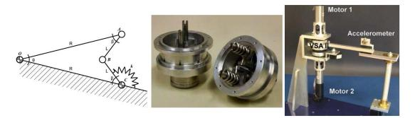
Figure 1.14. Functional scheme of VSA-II (4-bar transmission mechanism). Link OA is driven by a motor at O. The torque spring k is linear, while stiffness seen at O attains non-linearity through geometry (left); VSA-II prototype (middle); Test-bed for evaluation of VSA-II integration into a robotic joint (right).
