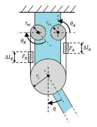
Figure 3.2. A classical representation of an antagonistically-actuated robot joint. Two motors, A and B, contribute equally to the overall joint torque and consequently move the joint, if their directions of rotation are opposite (for the adopted direction), whereas if the directions of motor rotation coincide, elastic elements co-contract and the joint stiffens.
