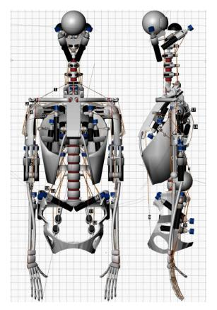
Figure 2.1. Front and side views of the complete anthropomimetic robot model implemented by Diamond et al. in [128]. The authors initially captured Eccerobot morphology and, accordingly, created a static CAD model. The model was then exploited in the Bullet physics engine with user-shaped constraints; complex kinematics dependencies, as well as compliant elements, were introduced.
