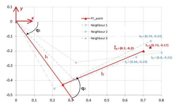
Figure 4.6. Two-DoF planar robot as a target system for estimating kinematic coefficients. The actual position  $(\hat{F}_0)$  and the desired position  $(F_0)$  of the hand tip are depicted by red triangles. The selected nearest neighbors  $S_1$ ,  $S_2$ , and  $S_3$  are marked by blue squares.
