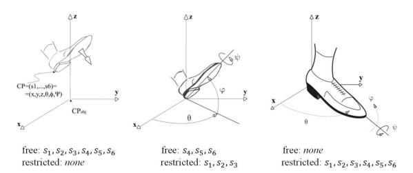
Figure 2.8. Identification of functional coordinates s – free and restricted. Impact occurs if any of the free coordinates reaches zero. Thereby the functional coordinate exchanges its set: from free to restricted functional coordinates. Each exchange between these sets requires a new corresponding mathematical model.
