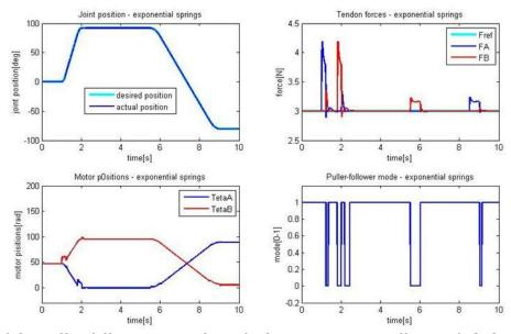
Figure 3.9. Puller-follower control applied to antagonistically-coupled drive using exponential springs as elastic elements (3.34), (3.35). Validation is demonstrated by trajectory tracking (top left); Force control in the antagonistic tendon (top right); The positions of motor A and motor B, whose simultaneous action ensures proper joint position and antagonistic force (bottom left); Changing of the roles of motor A and motor B as the follower, or vice-versa if mode 0 is active (bottom right).
