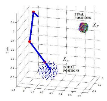
Figure 4.3. Spherical grids of initial and final hand-tip positions, formed in the experience acquisition stage. Sphere  $X_s$ , with a 0.1m radius and the center in the Cartesian point (0.2, -0.4, -0.45), captures all initial positions in the training phase. The final sphere  $X_f$ , with a 0.05m radius, located around Cartesian coordinates (0.55, -0.2, 0), consists of about 100 points from each of the initial positions within the sphere  $X_s$ .
