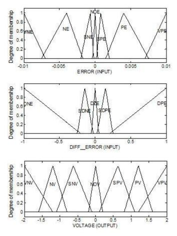
Figure 4.7. Fuzzy membership functions for two inputs (position error  $e_x$ , derivative of position error  $de_x$ ) and the output (voltage) for the x axis of the Cartesian frame. Analogous figures apply to y and z axes.
