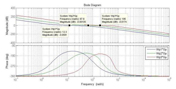
Figure 3.21. Loop-shaping procedure using pre-compensator  $W_p$  to reshape the target system of joint position control  $G_p$ . Three pre-compensators, resulting in different bandwidths, are selected. The ultimate controllers of different dynamics (bandwidths) are selected to cover all necessary joint dynamics requirements – from the beginning (high load, low frequency motion/disturbances) to the end of the kinematic chain (low load, high frequency motion/disturbances).
