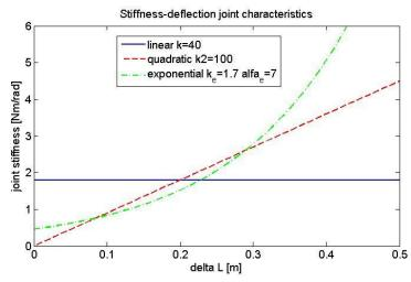
*Figure 3.11. Resulting stiffness-deflection dependence for an antagonistically-actuated joint with all three sources of compliance: linear, quadratic and exponential springs.*
