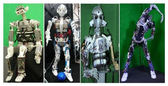
Figure 1.8. Evolution of anthropomimetic legged robots at JSK Lab of the University of Tokyo. From left to right: Kenta (2003), Kotaro/Kojiro (2006), Kenzoh (2010), and Kenshiro (2013).
