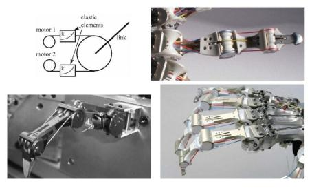
Figure 1.15. Functional scheme of antagonistic actuation employed in fingers of DLR Hand Arm System [83] (top left); First prototype of DLR anthropomorphic finger (bottom left); Second prototype of DLR anthropomorphic finger (top right); Assembled hand using antagonistic actuation for finger control (bottom right). Tendon routing was optimized to minimize friction and wear, while all drives of the hand were moved to the forearm to fit human size.
