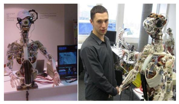
*Figure 1.1. Eccerobot - the pioneer among anthropomimetic robots, and a motivation for the work on the thesis.*
