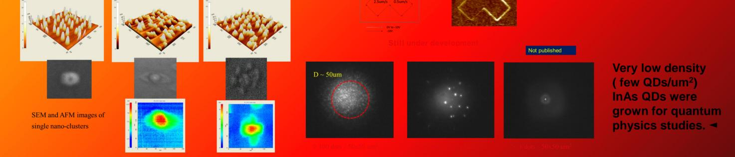
Conventional SK-mode grown In(Ga)As QDs are grown on GaAs, Si. These were used for solar cell, QDIP (IR sensor) etc.
