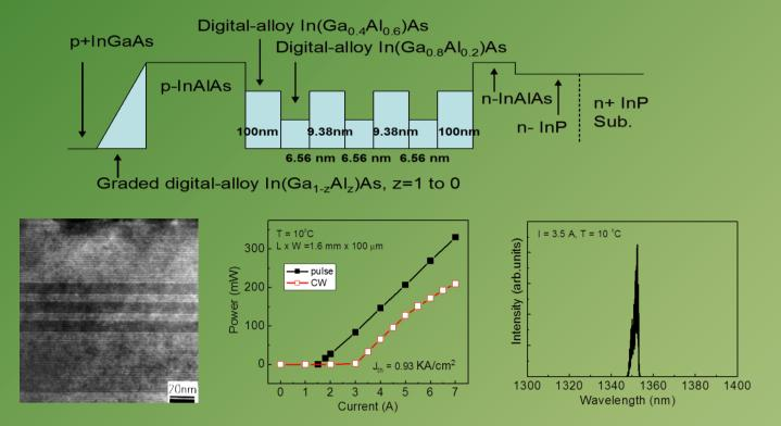
**Digital alloy InGaAIAs were grown by repetition of short period** superlattices of few monolayer thick-InGaAs and InAIAs.▲
