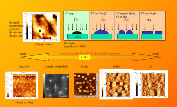
With GaAs/AlGaAs droplet QDs, we can grow QDs, Q-rings, Q-disks, and Q-pits. ▲
