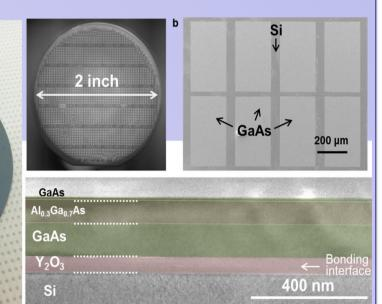
• Uniform wafer bonding using Y<sub>2</sub>O<sub>3</sub> layer • Wafer scalability up to 2 inch (machine limit)
