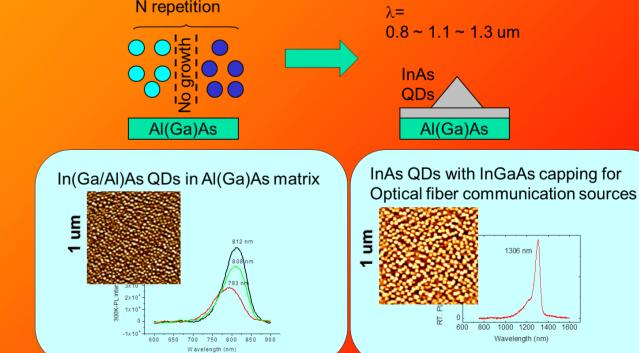
**MEE-mode grown** InAs, InGaAs QDs were used for 1.3um-LD, PD etc.
